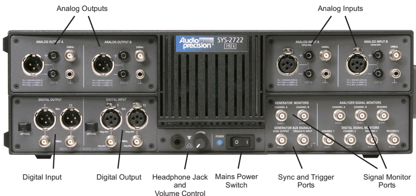
Figure 11. SYS-2722 front panel.
